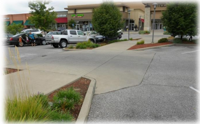
This raised crosswalk is traffic calming for both vehicles and pedestrians.
