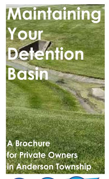
Your detention basin is a storm water best management practice (BMP) designed to temporarily capture and hold storm water runoff during periods of heavy rain.
